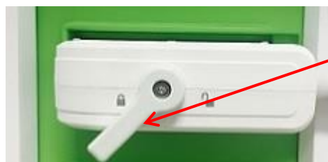
Figure 21: Transducer Connector Orientation
