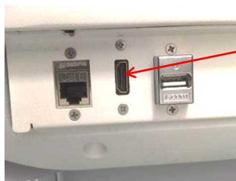
Figure 11: Second monitor output (HDMI) Connector
