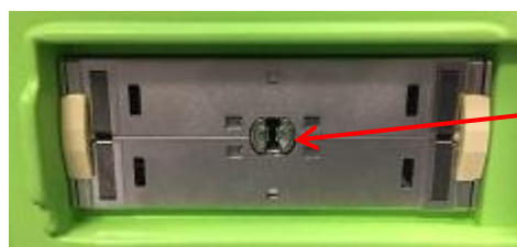
Figure 20: Lock Notch on the Transducer Connector Slot
